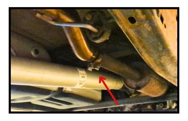
Step 3. Install the Inlet Pipe
