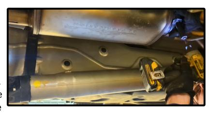
Step 4. Install the Over Axle and tailpipes using the supplied 2.5" clamps. Locate the welded hanger to the OEM rubber insulator. We have found it easier to unbolt the OEM isolator from the frame, slide it on the hanger, then bolt it back on while installing the tailpipe.
