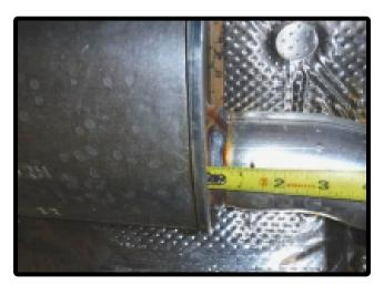
Step 5. Install the driver and passenger side muffler deletes using the supplied clamps, the clamps should only cover the slots and not be slid on to the solid part of the tube.
